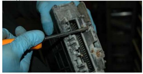
After moving the bracket remove the four T-15 torx screws.
