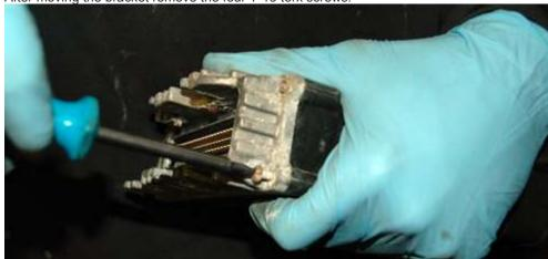
After removing the four torx screws, split the ECU case open. If the case has never been open before it may be difficult to open. A couple of taps with a screw driver around the edges usually helps.
