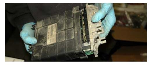
Reconnect the ECU and then the battery. Make sure the car starts before reinstalling the rain tray. When reconnecting the battery **MAKE SURE THE KEY IS OUT OF THE IGNITION.**After connecting the battery put the key in the on position (position before start) and let the throttle body adapt. You will hear the throttle body whine. Once the whining stops you can start the car.
