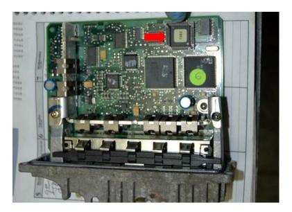
Carefully use a pick or a thumbtack to remove the old chip
