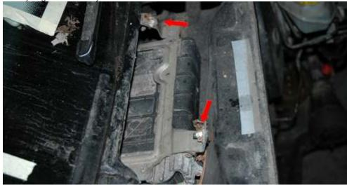
After you remove the two bolts, slide the bracket towards the passenger side then out. Next, push/pull the harness connector up.
