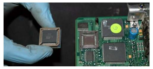
**Carefully** install the new chip, making sure all the pins are lined up before you push it in. The chip can ONLY go in one way. Make sure to line up the corner with the angle on it.
